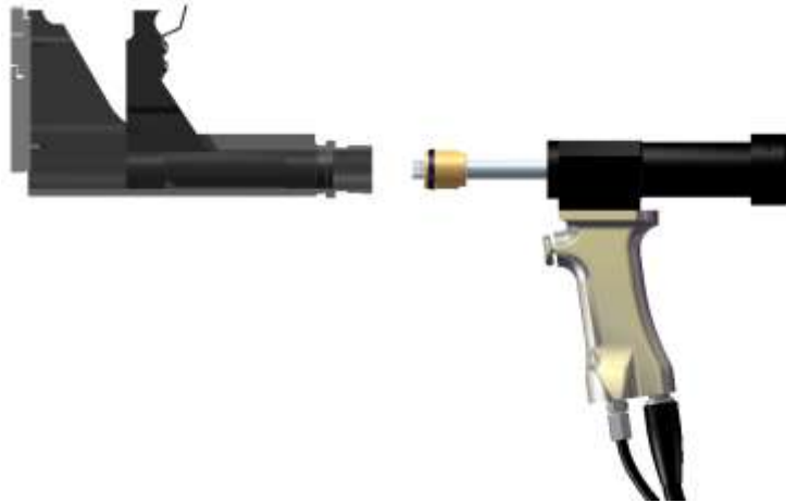
Figure 5-1 Little Brute Piston Rod and Slide Assembly, Threaded Mandrel (Guard not shown for clarity)
