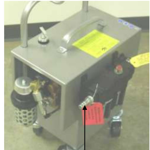
Figure 2.0-2 Location of Air Disconnect
