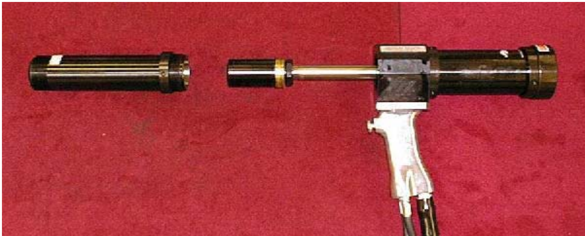
Figure 4 MB-30 Barrel Removed
