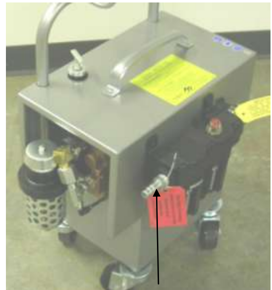
Figure 2.0-2 Location of Air Disconnect
