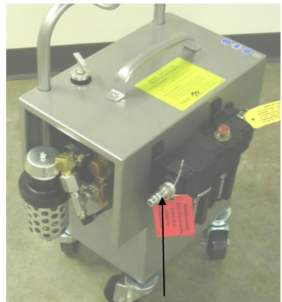
Figure 2.0-2 Location of Air Disconnect
