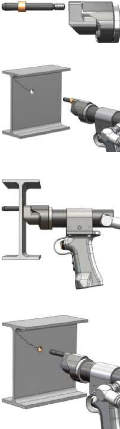
Place bushing onto the back end of mandrel. Insert the mandrel through the jaw and thread into adapter.
