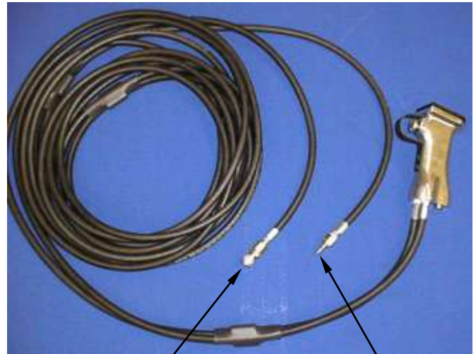
Figure 3.1.2-2 Trigger Assembly with Hoses
