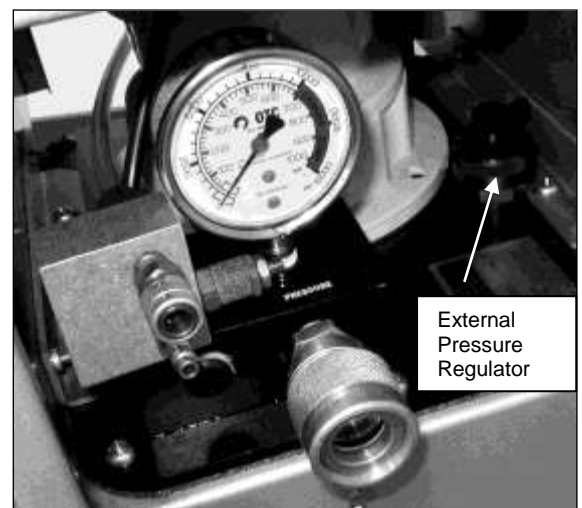
Figure 3.3-1 PowerPak Pressure Adjustment
