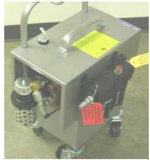
Figure 2.0-2 Location of Air Disconnect
