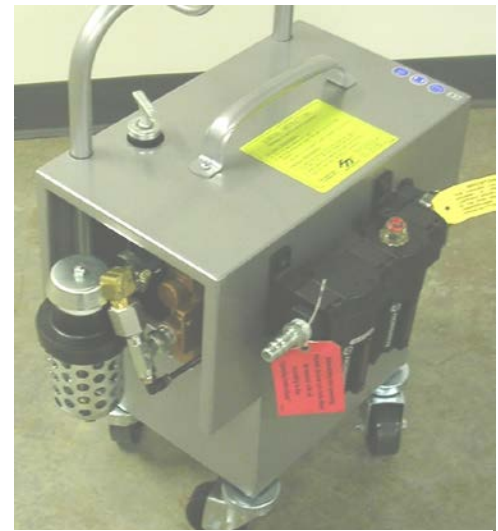
Figure 2.0-2 Location of Air Disconnect
