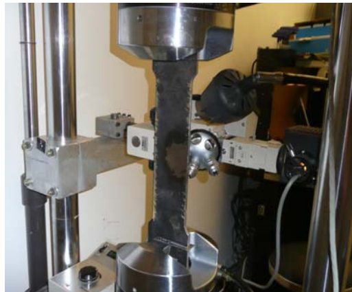
Figure 6. MTS Test Machine Fitted with Hydraulic Grips and an Optical Microscope
