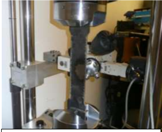
Figure 5. MTS Test Machine Fitted with Hydraulic Grips and an Optical Microscope
