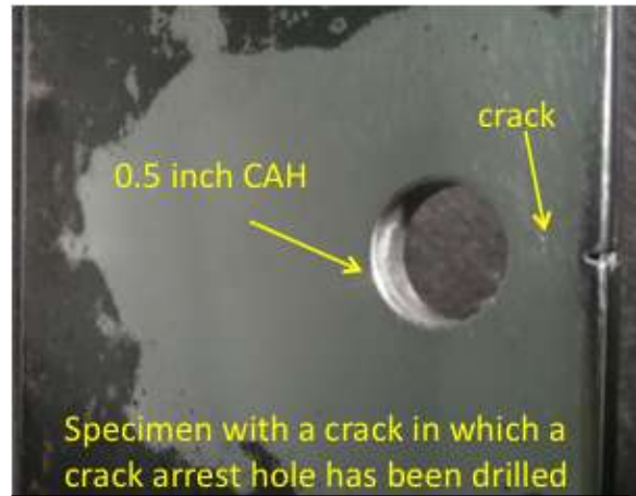
Figure 7. Picture of a CAH Repaired Crack
