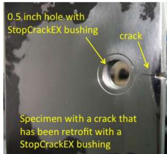
Figure 8. Picture of a StopCrackEX Repaired Crack
