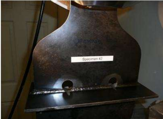
Figure 13. Simulated Welded Flange Coupon with Crack Arrest Holes at Each End of Crack
