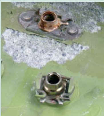
AIRCRAFT CARGO SIDE PANEL (Top: Riveted nut plate / Bottom: ForceTec)
