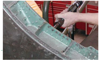
Reworking damaged riveted nut plate holes with ForceTec.
