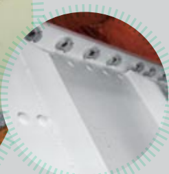
ForceTec retainers installed in cargo aircraft floor rails.
