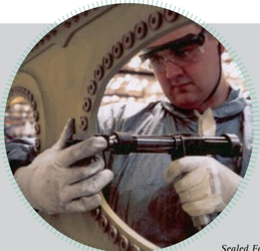
Sealed ForceTec in a wing access panel mounting.
