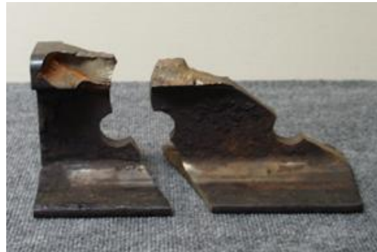
Figure 2. Example of Separated Piece of Track End
