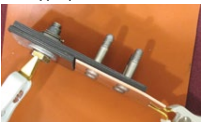
Expanded Nut Plate, Blind Nut, and Bushing electrical conductivity comparison with a net fit, hex-nut NAS fastener.
