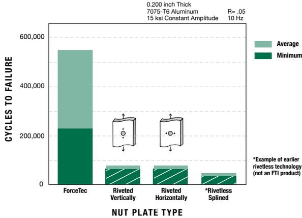
Installation of ForceTec cold expands the fastener hole to increase the fatigue life of the installation plus it eliminates attachment rivet holes and other induced stress risers. (FTI Report #33820)
