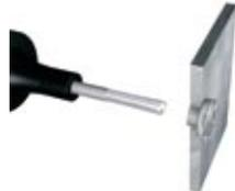
**Insert the mandrel/sleeve assembly through the retainer**
