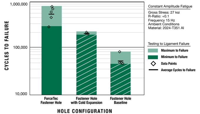
ForceTec provides additional benefit over coldworked nut plate fastener holes by protecting the hole with an interference fit "bushing." (FTI Report #83823)
