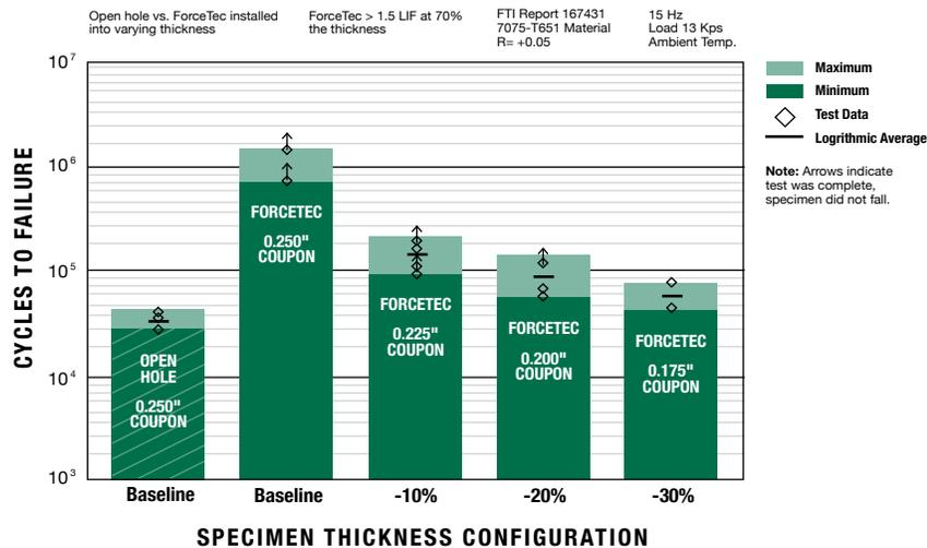
*A 0.250" thick, open hole specimen was tested against four different thickness sized ForceTec specimens using the same load and ever increasing net section stress. The results showed that ForceTec in a 0.175" thick coupon achieved a service life greater than the baseline specimen life. This is a reduction of 0.075" or 30% of the baseline specimen thickness. (FTI Report #167431)*
