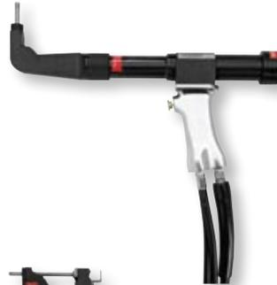
*Right Angle Puller for holes in pockets or areas with limited front-side access.*
