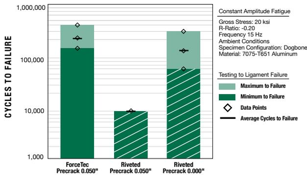
Damage tolerance testing with 1/4" nut plates showed ForceTec installed with a 0.050" pre-crack performed better than an un-cracked riveted nut plate installation. (FTI Report #89408)
