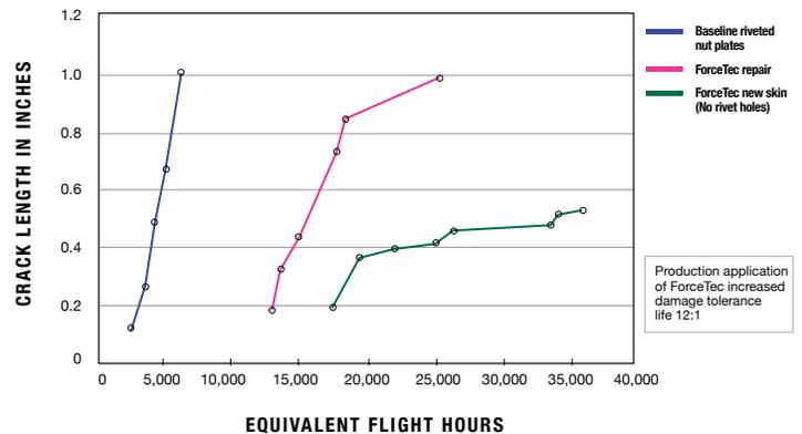
Replacement of riveted nut plates with ForceTec to remove fatigue cracks on fighter aircraft access panel door attachments extended the life over 7:1. (FTI Report #85874)
