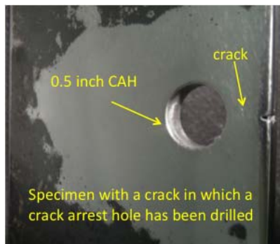
Figure 4: CAH repaired crack
