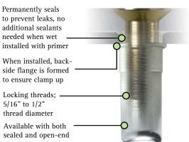
The mechanical expansion provides a secure, permanent sealing in applications where sealing is required. Unlike competitive products, the nut is installed without the need for machining complex elliptical countersinks or the need for special surface preparation.
